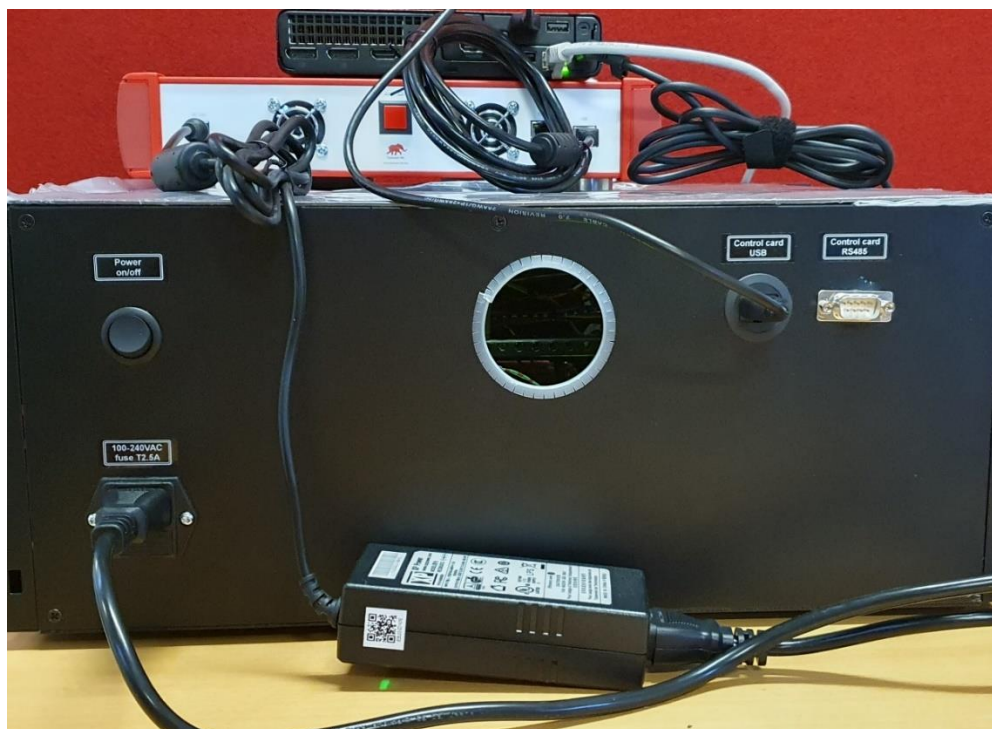
Figure 3: Rear with connection for mains, USB and RS485 for control board.
