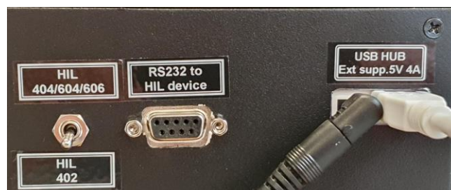
Figure 8: Selector between HIL402 and HIL404/604/606 devices and RS232 port for serial communication.
