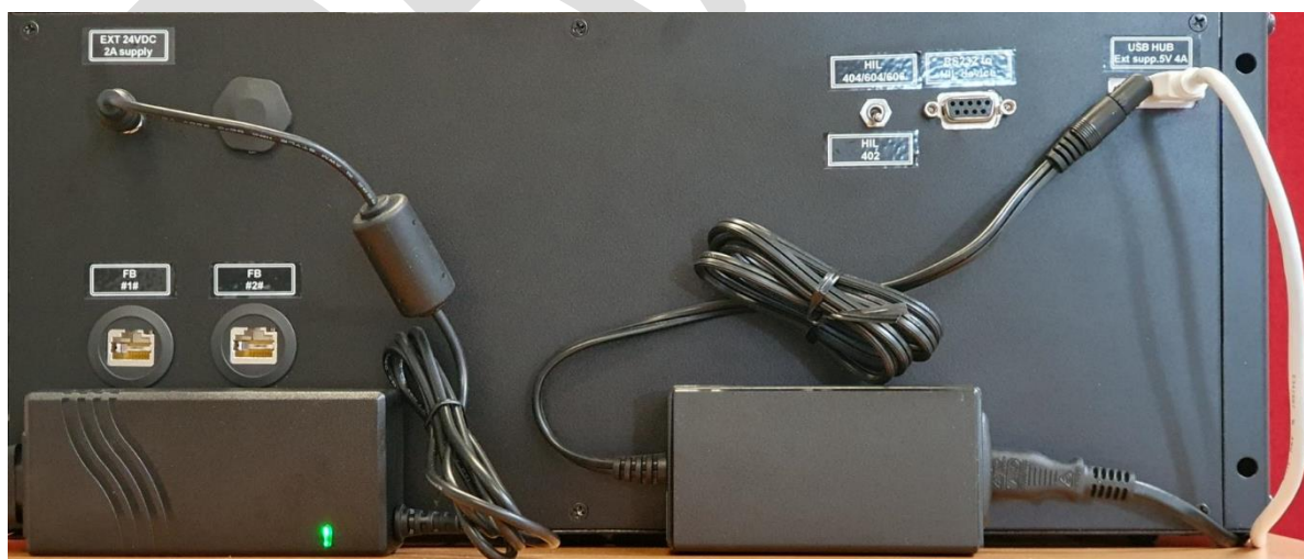
Figure 7: Rear with connection for main power supplies, USB for access to the service-port of iC7 control unit, Ethernet based Fieldbus for control unit and serial communication with HIL404 device.
