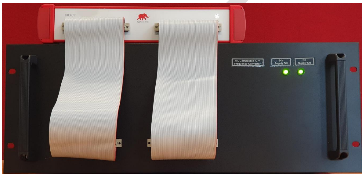
Figure 6: Front with ribbon-cables to HIL402 device.
